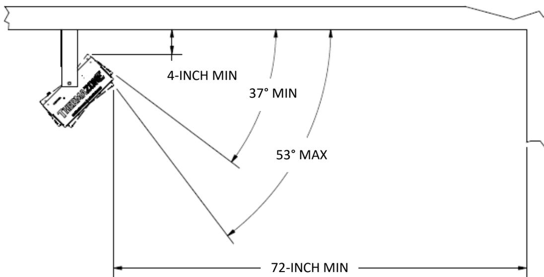
**Fig. 4 – CEILING MOUNTING ANGLED TOWARDS VERTICAL SURFACE**
