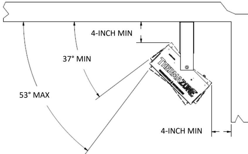
**Fig. 3 – CEILING MOUNTING ANGLED AWAY FROM VERTICAL SURFACE**
