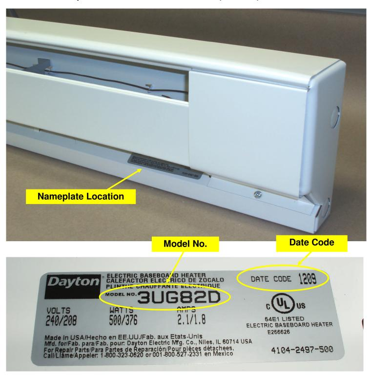
If Model 3UG82D <u>AND</u> Date Code 1209, go to step 3. If not this model or date code, heater is not affected by this recall.
