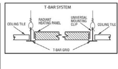
NOTE: Heating panels do not have a fire or hazardous rating, but construction is of fire retardant materials. Panels normally are treated like light fixtures. If necessary, acoustical tile can be placed on top of the panels.
