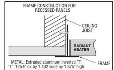
NOTE: Heating panels do not have a fire or hazardous rating, but construction is of fire retardant materials. Panels normally are treated like light fixtures. If necessary, acoustical tile can be placed on top of the panels.
