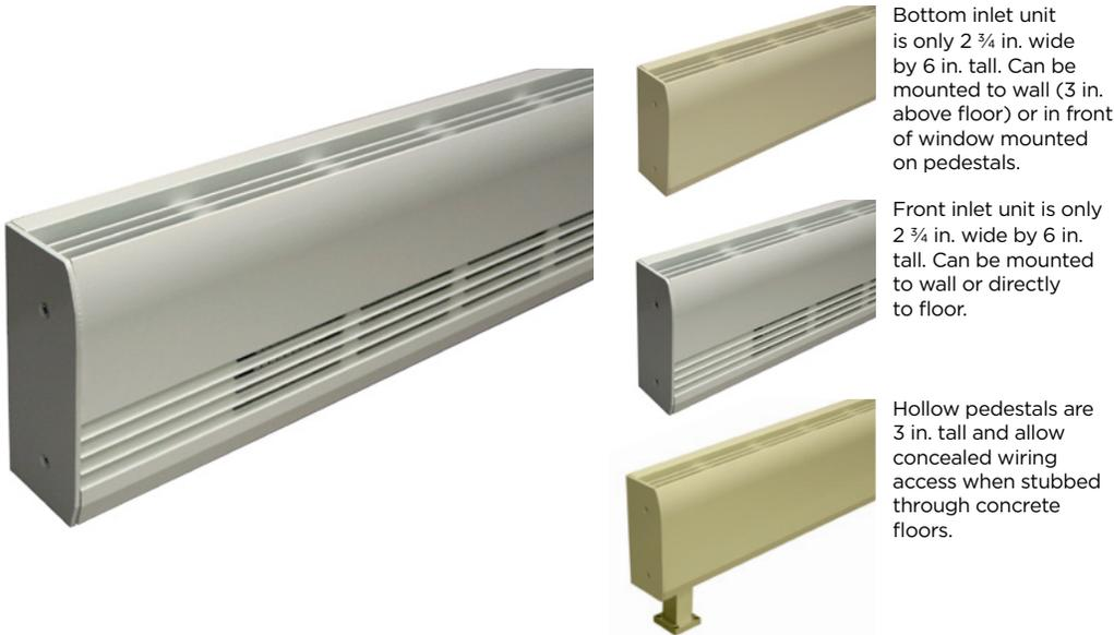
Bottom inlet unit is only 2 ¾ in. wide by 6 in. tall. Can be mounted to wall (3 in. above floor) or in front of window mounted on pedestals.
