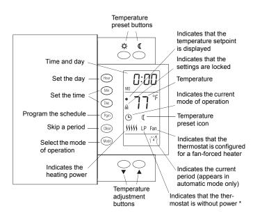
\* LP appears only for the first two minutes when the thermostat is without power. This can occur during a power outage or when the thermal protection device inside the base-board heater is opened.
