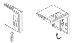
Make the appropriate connections. Please note that the thermostat wires are non-polarized; either wire can be connected to either terminal.
