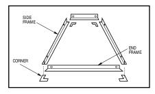
FRAME CONSTRUCTION FOR RECESSED PANELS
